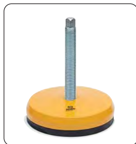
Part. R0406 - Pag. R55 Ø 123 • Painted steel • Max. load 50000 N.
