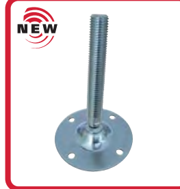
Part. R0349 - Pag. R42 Ø 123 • N. 4 holes • Stainless steel and zinc plated steel • Max. load 10000 N.
